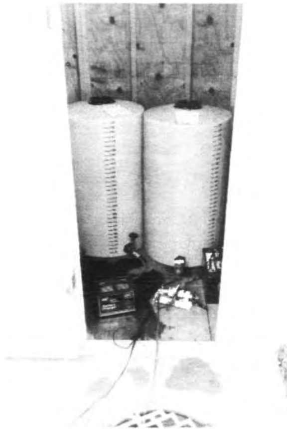
Figure 7. Dye injection system
