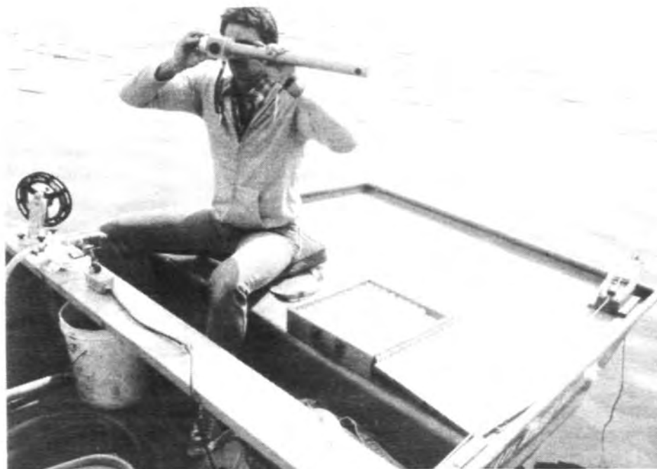
Figure 5. Lining up on transect stakes using the range finder
